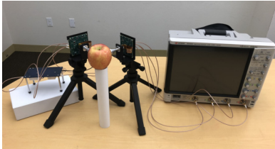
Figure 12: Our 60 GHz mmWave testbed setup showing how we measure signal reflection from a fruit
